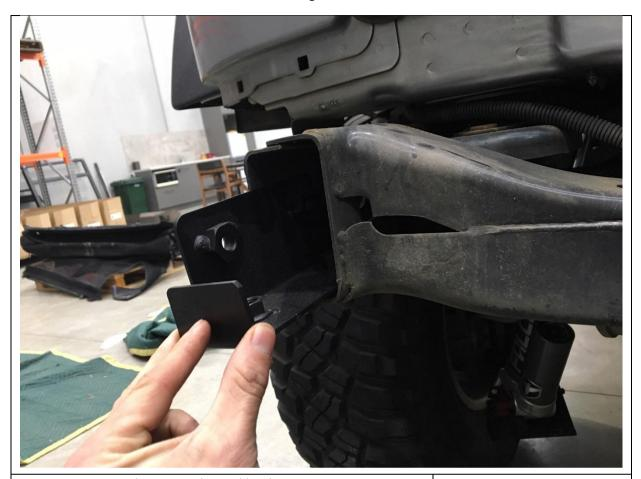
8. Insert nut plates into chassis like shown.
