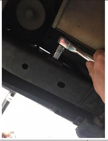
4. While still underneath remove 2 x M10 bolts as shown, and loosen M10 bolts further up on same bracket
